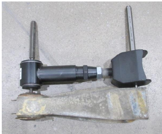
Figure 5 - Detroit Speed vs. Stock Upper Link
