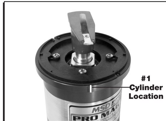
Figure 3 Positioning the Rotor Tip.
