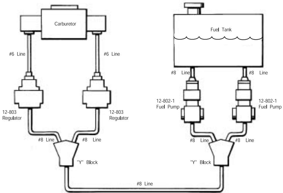
Figure 4 – One (1) #12-706-1 VOLUMAX pump feeding dual carburetors.
