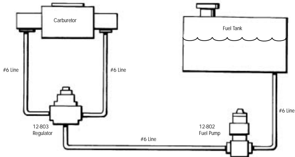
Figure 2 - One (1) #12-706-1 VOLUMAX pump feeding single carburetor.
