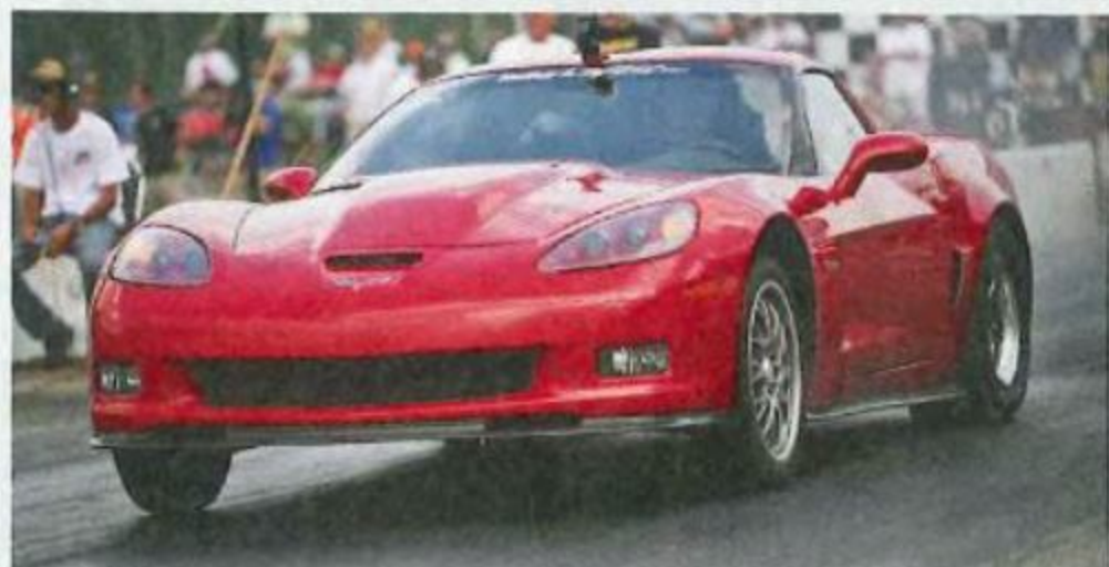
TJ Strange of RPM Transmissions was one of the most interesting entrants to SAM All Motor, a big hydraulic roller spins this Z06's LS7 with an RPM 6060 and 4.10 rear. TJ went to base Corvette rear brakes to fit the Weld 15x10 wheels and Hoosier 275 radials. When he gets the slipper clutch figured out, this should be a 9-second ride fit for the street. Unfortunately, a few issues kept him in the mid 10s.
