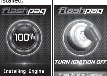
**STEP 10** - Turn the ignition Off. STEP 11 - Press OK to return to the main menu.
