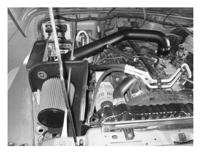
**STEP 20 -** Remove the temperature sensor from the OE tube and insert it into the grommet on the intake tube and connect the harness to the sensor.
