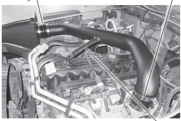
**STEP 16 -** Install the intake tube into the couplers, align the tube then tightencoupler clamps.
