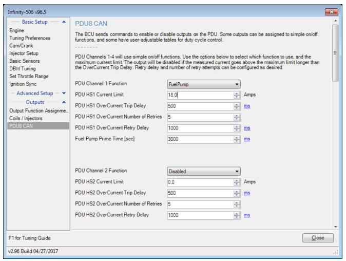
In the screenshot above, The HS1 output will turn off if the measured current is above 18.0 amps for 500ms (0.50 seconds). The output will stay off for 1000ms (1.0 second) and then retry. The output will only retry 5 times, after the fifth overcurrent event it will stay off until the ECU turns off and restarts.
