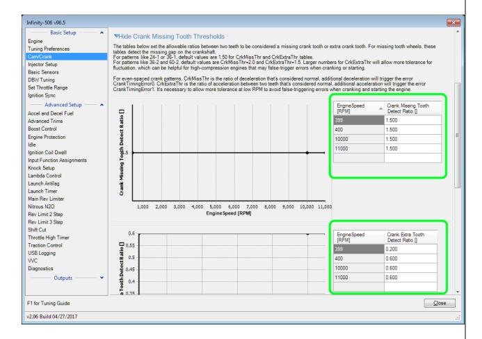
6. Cam Error Ignore function, to use the cam signal for sync at low RPM but ignore noisy cam signals at high RPM. If the CrkMissThr and CrkExtraThr tables are configured to detect crank errors, it can be safe to ignore cam errors at high RPM.
