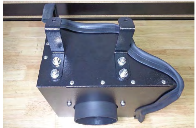
16. Attach the 2 brackets (15) to the heat shield as shown, using ¼-20 screws (10) (against the heat shield), and flat washers (12), lock washers (11), and nuts (16) (against the brackets).
