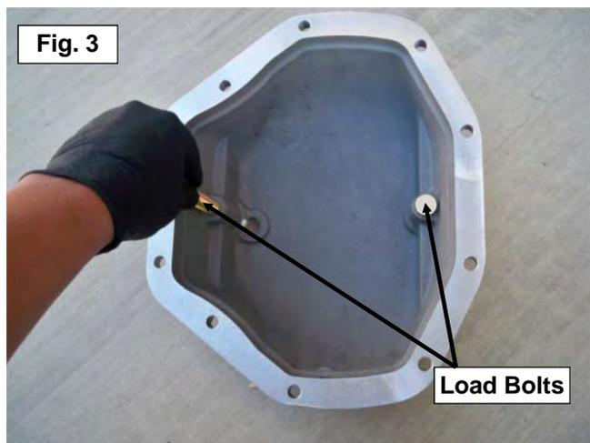
12. Install the rest of the supplied bolts and washers and torque to 25 ft/lb. in a crisscross pattern.
