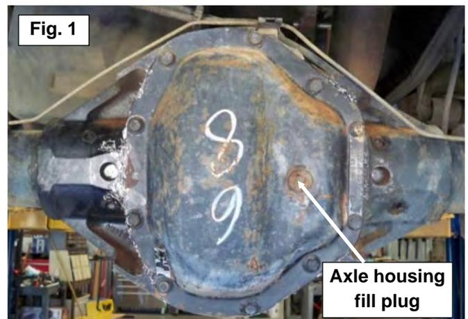
5. Carefully pry the cover loose with a flat head screw driver, being careful not to damage the surface, and allow the oil to drain. Remove the last bolt and the cover once completely drained.
