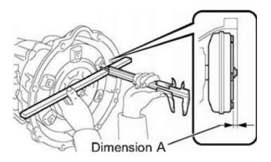
A. Measure Dimension A: While holding the torque converter in place against the transmission, use a straightedge to measure the distance between the bell housing mating surface and the torque converter mounting pads.
