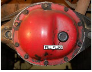
4. Carefully pry the cover loose with a flat head screw driver, being careful not to damage the surface, and allow the oil to drain.
