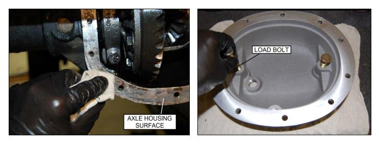
11. Install the rest of the supplied bolts and washers and torque to 15 ft/lb. in a crisscross pattern.
