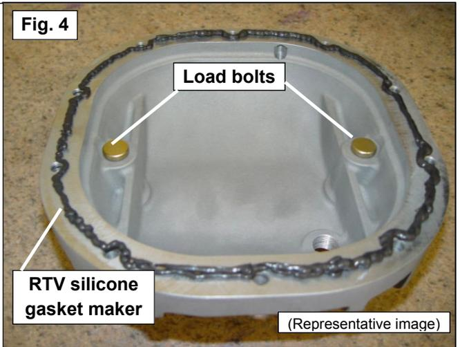
12. Install the B&M Differential Cover on the axle housing using a supplied bolt and washer at a bottom hole on the cover so it can be used as a guide.
