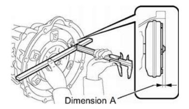
A. Measure Dimension A: While holding the torque converter in place against the transmission, use a straightedge to measure the distance between the bell housing mating surface and the torque converter mounting pads. (Typical C6 torque converter depth = 1-1/8", ±0.050".)
