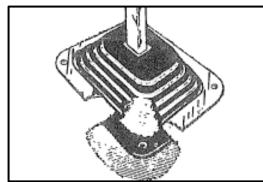
5. Slip bottom boot lip under carpet. Place hold-down plate into position and fasten with sheet metal screws supplied. Remove protective paper on chrome side of holddown plate.
