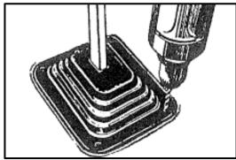
4. Replace boot. Drill 1/8" diameter holes through floor using boot holes to locate hole positions.
