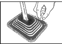
1. Remove knob. Slip boot over stick and down to floor. Use chalk to trace the outline of the boot on to the carpet.
