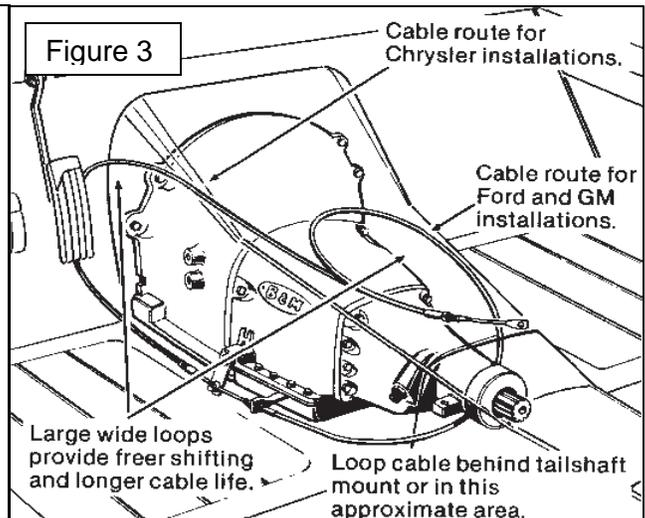
STEP 4. Move the transmission selector lever by hand to the full rear position (LOW). Place the shifter lever to the LOW gear position (all the way back). Adjust the large nuts on the cable so that the swivel will slide into the front ("F") hole on the selector lever. Tighten the large nuts completely. Be sure that the swivel will slide freely in and out of the "F" hole in the selector lever.
