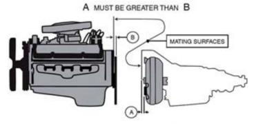
C. Verify that Dimension A is greater than Dimension B. If it is not, the torque converter is not fully seated. Pull it off slightly, then, while rotating it, push it back on. Continue to do this until you feel the torque converter move inward and make the proper engagement. Then repeat and compare Dimensions A and B. Do not proceed further until the torque converter is fully seated.
