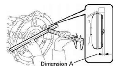
**A. Measure Dimension A:** While holding the torque converter in place against the transmission, use a straightedge to measure the distance between the
