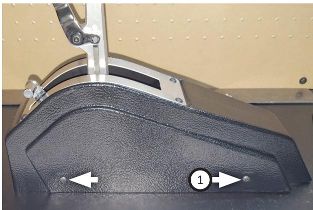
10. Place console over shifter and attach to mounting plate using (x4) **screws (1)**. Thread knob onto shifter stick, turn to desired position and tighten jam nut against knob.
