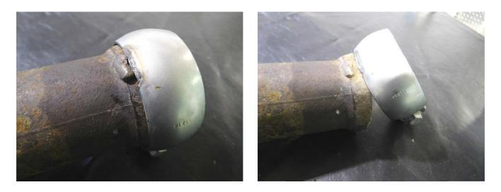
3) Place a factory clamp onto one of the new Flowmaster tips and put up into position behind the resonator on the right tailpipe. Tighten the clamp enough to hold the tip in place and adjust to the desired position. Tighten the clamp securely. Repeat this step on the left side of the vehicle.
