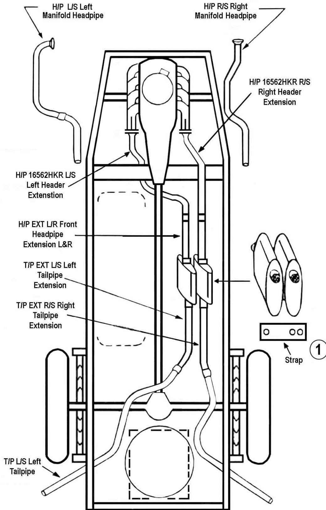
**1** Install mufflers side by side in this position with center inlet in front. Use 3-hole straps & U-clamps for proper clearance between mufflers & pipes.
