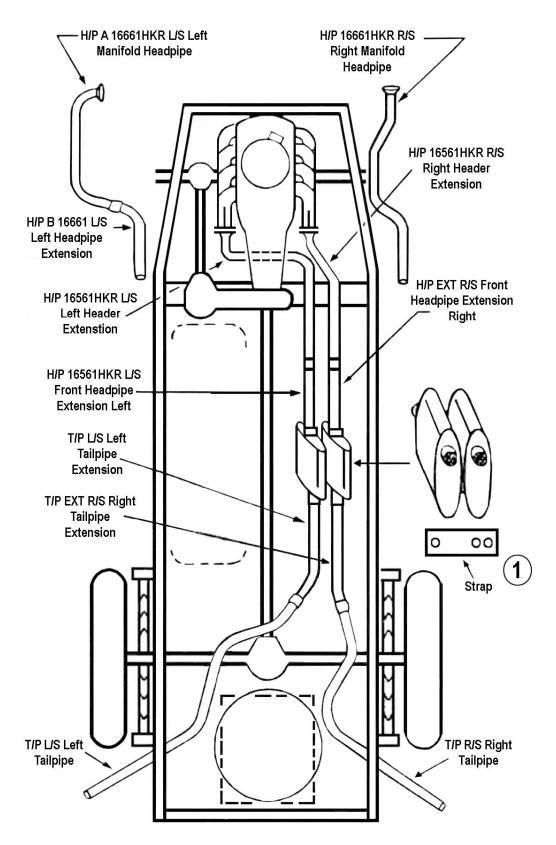
Install mufflers side by side in this position with center inlet in front. Use 3-hole straps & U-clamps for proper clearance between mufflers & pipes.
