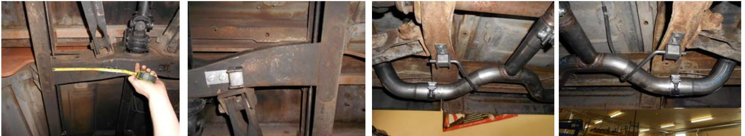
2) Take the right and left H-pipe assemblies, **86074 & 86075** and connect them together at the center cross-over connection. Place them up into position and connect the hangers on the pipe to the rubber mounts installed above. The hanger rods should stick thru the rubber block on the **HA572** hanger approx. 1.00". Support the front of the assembly with a stand. Place the provided 2" clamp at the center H-pipe connection.
