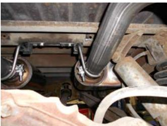
6) Place a supplied clamp onto the right muffler outlet; take the right over-axle tailpipe **#86077** and slide into the muffler outlet while connecting the front hanger on the pipe to the rubber mount installed in step 3 above. The tailpipes have been left long to work for long bed model trucks, for short bed trucks the rear of the tailpipes will need to be trimmed approximately 12.00". Place a second **HA572** hanger onto the rear hangers in preparation for the two steps below.
