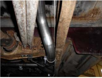
4) Take the **86076** muffler inlet pipes and place a supplied  $2\frac{1}{2}$ " clamp onto the expanded end, place them onto the back of the H-pipe assembly's **86074** & **86075**. Rotate them up into their approximate position and tighten the clamps enough to hold but still allow for adjustment.
