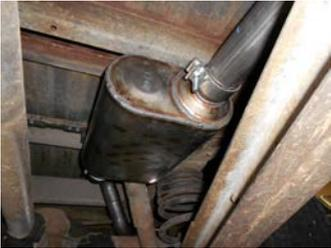
5) Take one of the **942548** mufflers and place a supplied clamp onto the inlet, slide the inlet onto the back of one of the **86076** inlet pipes with the outlet of the muffler in the center of the vehicle. Support the muffler with a stand and tighten the clamp enough to hold but still allow for adjustment.
