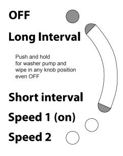
This diagram shows the detent positions of all Scott Drake interval wiper switches. The detent positions are felt as the wiper knob is rotated.
