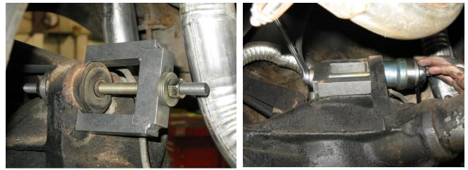
Figure 1 - Bushing removal
