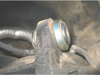
Figure 3 – Replacement Bushing Installed
