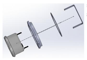
Assemble the fuel / oil pressure gauge as shown. Use (2) 8-32 lockunuts to secure the mounting bracket.
