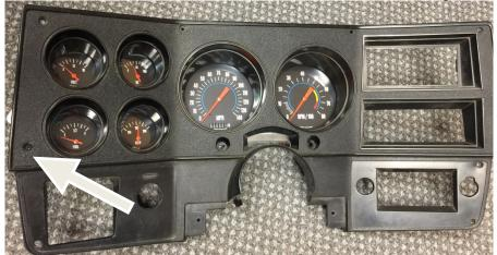
b. Due to differences in dash bezels from year to year, the upper aluminum standoffs are adjustable. Loosen these from the cluster and adjust them to fit the bezel. Use the black screws provided to secure the bezel to the aluminum standoffs.
