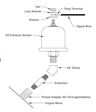
Use the 2 piece bushing kit provided to allow the sender to be mounted at a 45-degree angle pointing towards the driver's knees. This allows the sender to clear the back of the intake manifold, the underside of the distributor housing and also the firewall.
