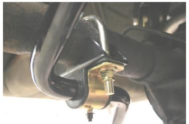
Figure 4 - Anti-Roll Bar Mounted on Rear Axle
