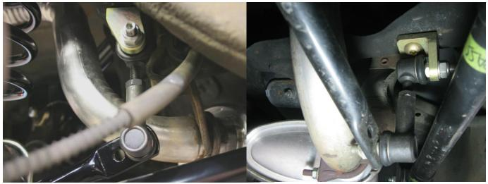
Figure 2 - Upper Mounting Bracket Orientation (Passenger Side Shown)
