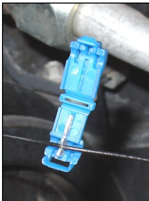
Figure 4 (T-Tap connector installation)
