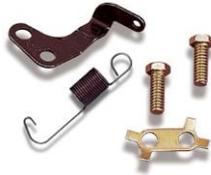
This is the hardware kit needed when installing a Holley universal carburetor with two mounting holes to a Ford with Automatic Transmission.
