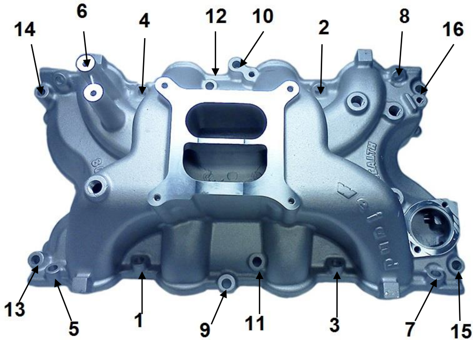
Figure 1 Bolt tightening sequence
