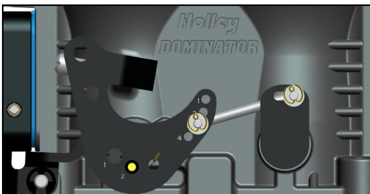
Figure 8 – Linkage shown from factory – progressive style actuation
