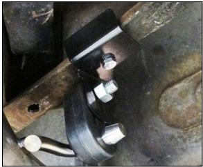
Figure 3 – Left tailpipe hanger bracket
