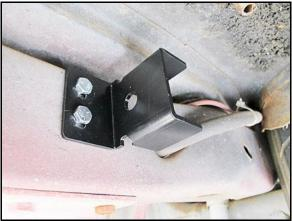
Figure 6 – Right tailpipe hanger bracket orientation
