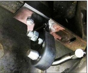
Figure 4 – Right tailpipe hanger bracket
