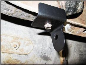
Figure 2 – Right over-axle hanger bracket
