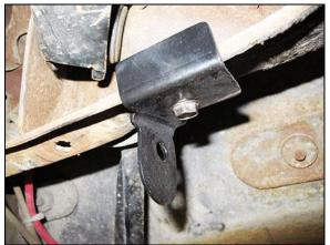
Figure 1 – Left over-axle hanger bracket
