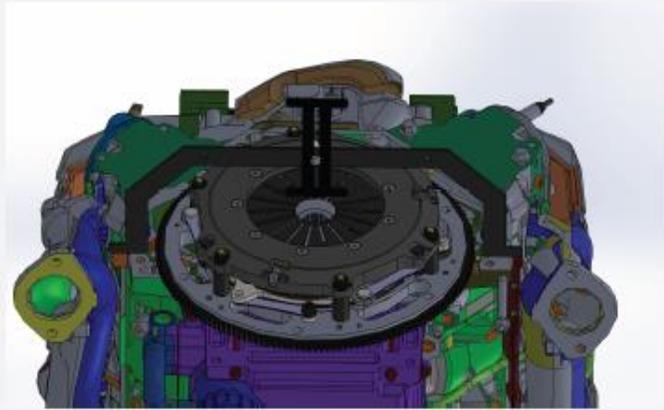
3. Slide locator toward clutch diaphragm fingers where the release bearing will ride. Tighten thumb screw.
