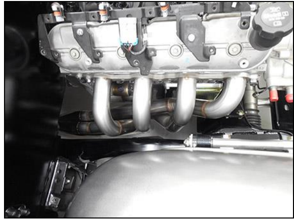
Right header installed
