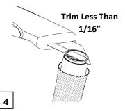
Trim the hose to be flush and square with the olive using a sharp blade.
