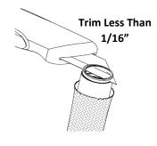
Trim the hose to be flush and square with the olive using a sharp blade.
