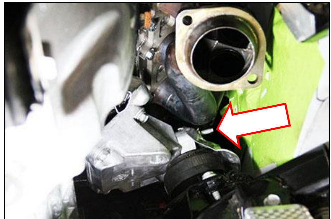
Figure 4 – Engine mount bolts
