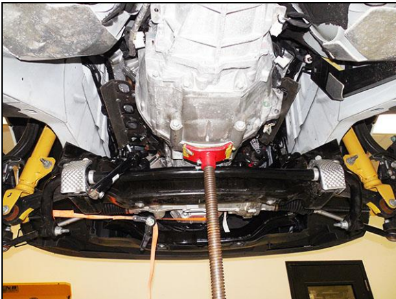
Figure 3 – Engine support and tie strap
