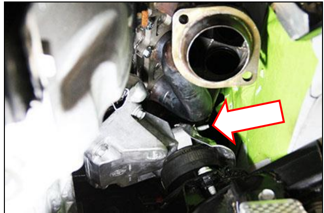
Figure 4 – Engine mount bolts
