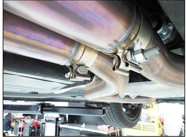
Figure 2 – Down pipe to X-pipe clamps
