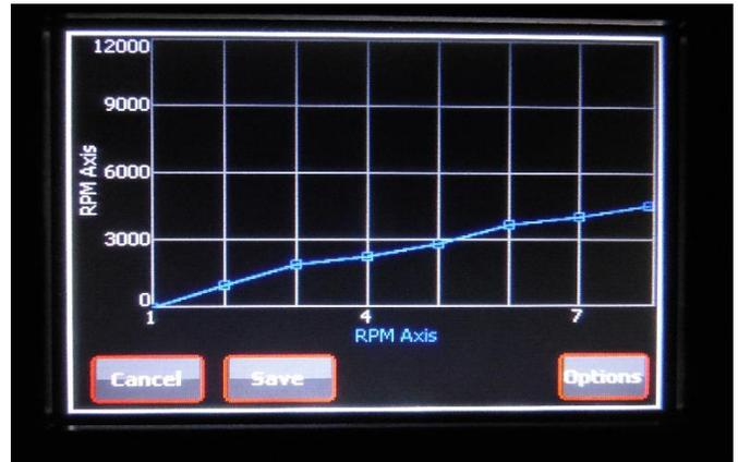
Figure 29 – MAP RPM Axis Table
