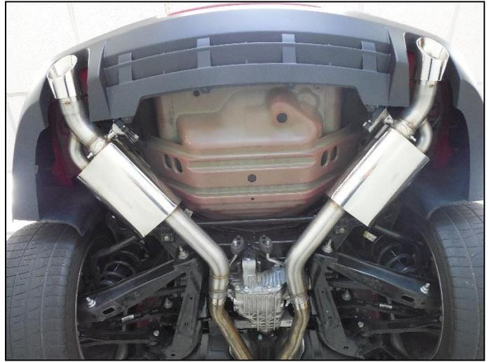
**Figure 2 – Dual tip rear mount installation**
