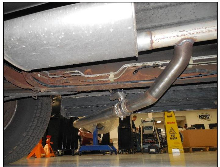
**Figure 4 – Side exit secondary cut out**
