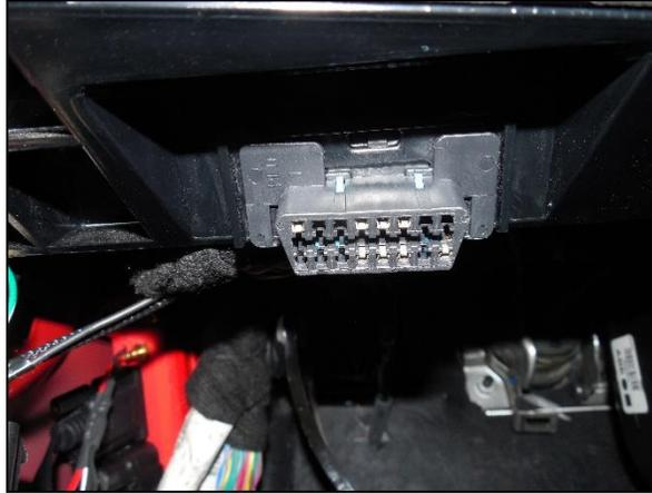
**Figure 9 – OBDII Connector**
