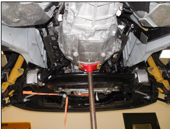
Figure 3 – Engine support and tie strap
