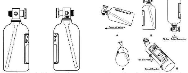
Figure 2 Nitrous Bottle Siphon Tube Orientation
