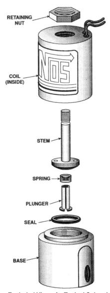
**Exploded View of a Typical Solenoid**
