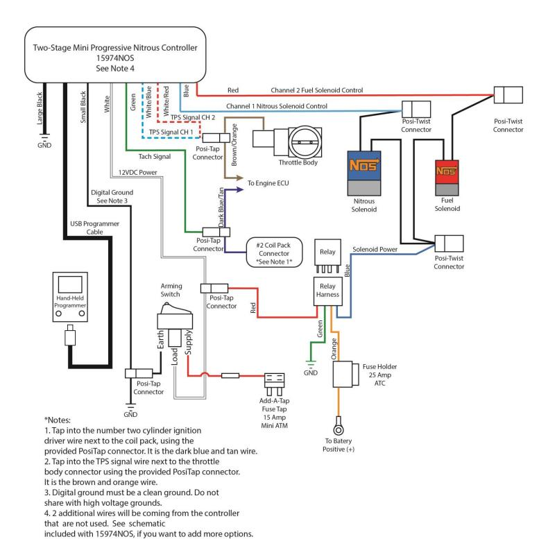
Figure 11 Electric Wiring Diagram
