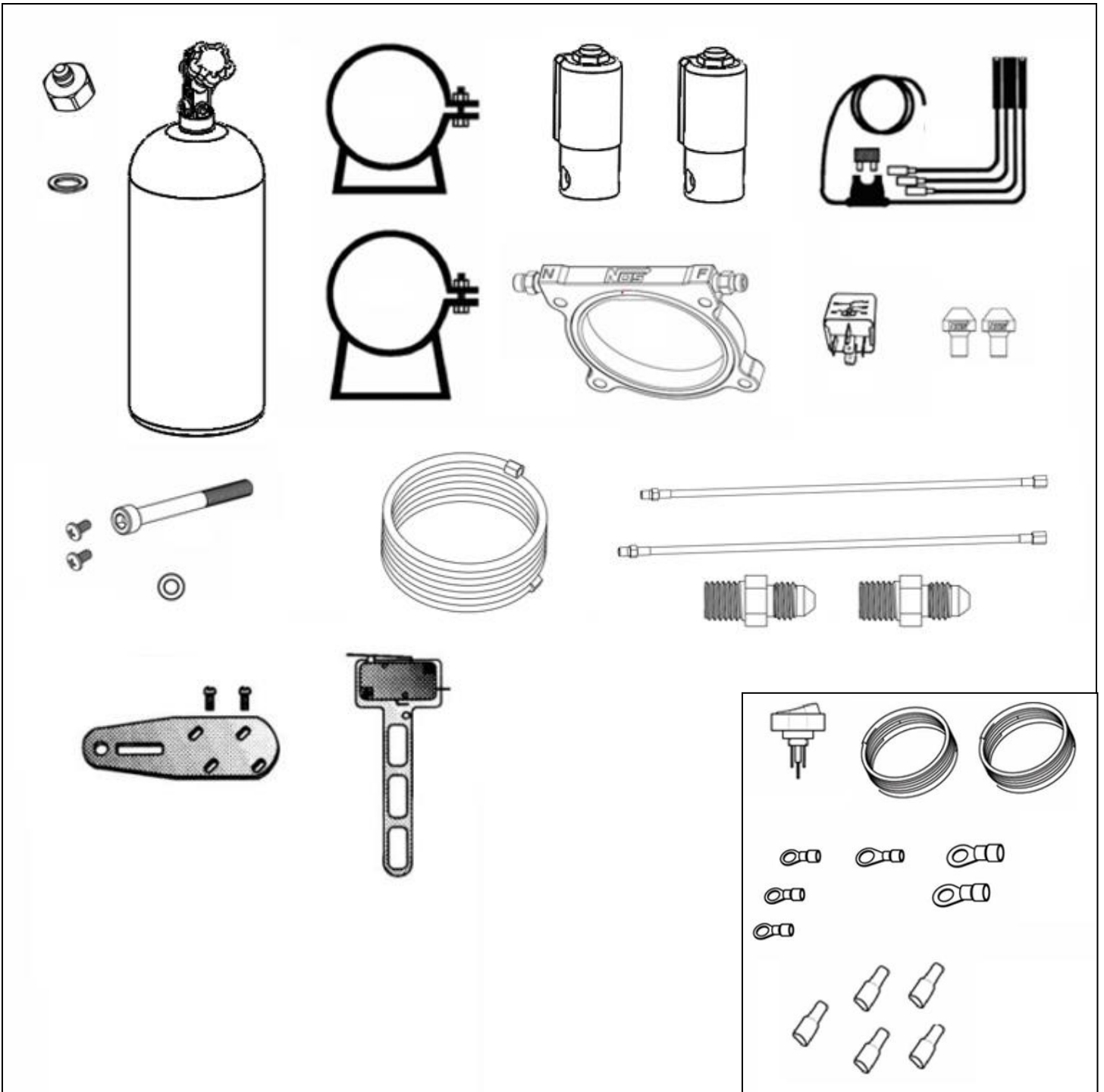
Figure 1 Kit Number 07166NOS Component Identification
