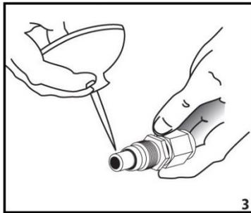
3. Lubricate the inside of the hose, the nipple threads and the socket threads with Earl's Assembly Lube or Engine Oil. Place the nipple in a vise.
