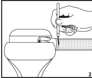
2. Place the socket in a vise and insert the end of the hose into the socket until the hose butts against the bottom of the threads. Gently pull the hose back until there is a 1/16" to 1/8" gap between the end of the hose and the bottom of the socket—mark hose at bottom of socket with a felt pen so that you can detect any tendency of the hose to be pushed out as you complete the assembly.
