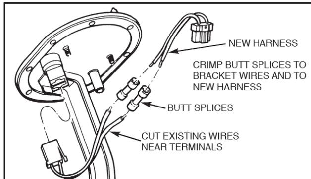
Some pumps will require removal of a protective rubber boot over the terminals, cutting the wires near the existing connector or terminals, and strip-ping 1/4" of insulation from the wires. Using the recommended tool shown in Fig. 6, crimp the butt splices to the bracket wires and to the new wiring assembly, making sure proper polarity is maintained. Snap the electrical connector into the pump.
