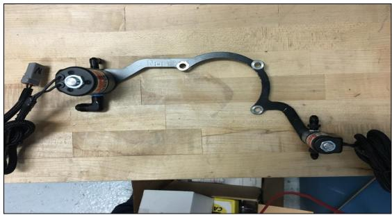
Figure 6 - Solenoid Bracket Assembly
