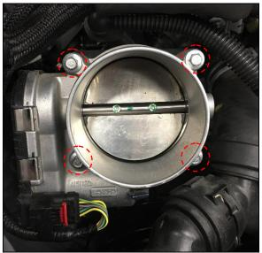
Figure 9 - Throttle Body Removal
