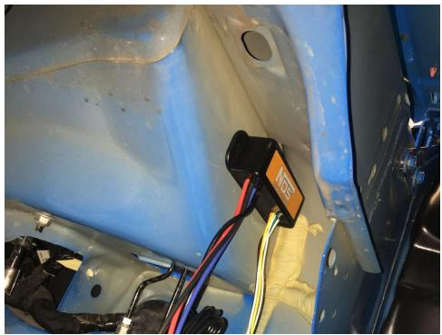
Figure 16 - Mini 2-Stage Mounting Location
