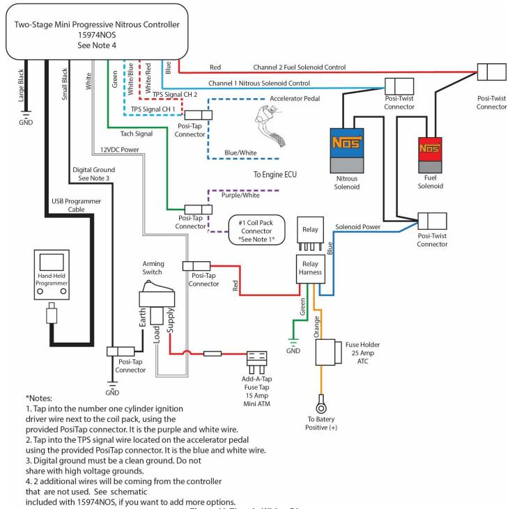
Figure 20 Electric Wiring Diagram
