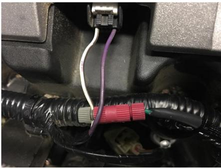
Figure 18 - Tach Signal Wire Connection
