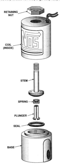
Figure 23 - Exploded View of a Typical Solenoid
