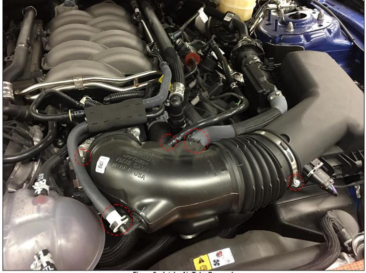
Figure 8 - Intake Air Tube Removal
