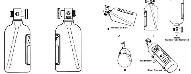
**Figure 2 Nitrous Bottle Siphon Tube Orientation**
