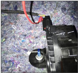
Figure 19 - TPS Signal Wires Connection
