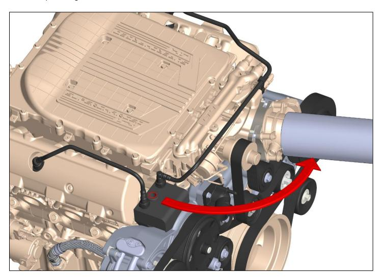
Air intake tubes vary in swap applications. The separator tank's vent plumbing will be custom for your specific situation. Earl's 90 degree 1/2" NPT to male -6 AN adapter (P/N AT982268ERL) can be used to adapt the tank vent to standard AN.
