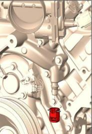
If ONLY installing the Holley ADD-ON power steering to wet sump applications, install the supplied red cap to the water pump barb. After installation, rotate the cap until the text is forward. See APPENDIX for alternate oil cooler plumbing.
