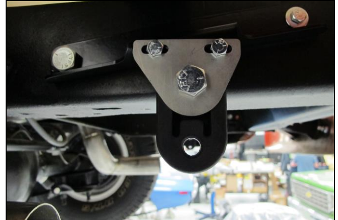
Driver's Side Dual Rear Exit System Tailpipe Hanger Installation Figure 3
