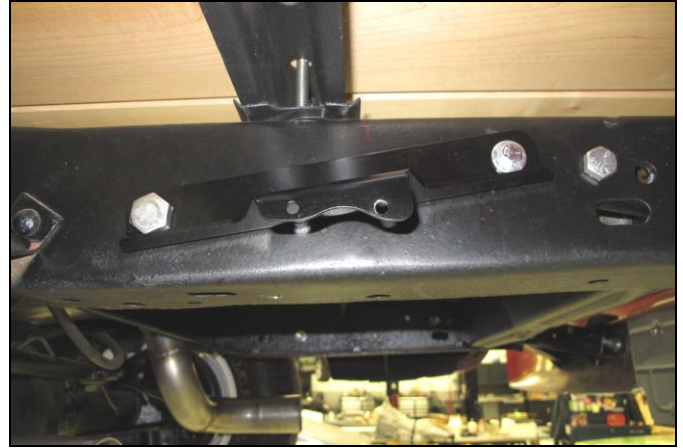
Driver's Side Tailpipe Hanger Frame Bracket Installation Figure 2
