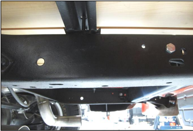
Driver's Side Tailpipe Hanger Frame Bracket Installation Figure 2
