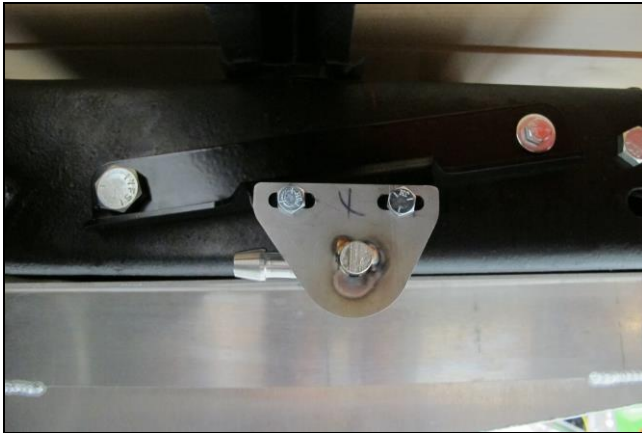
Driver's Side Dual Side Exit System Tailpipe Hanger Installation
