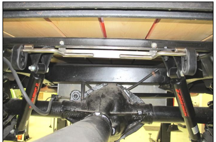
Front Tailpipe Hanger Frame Bracket Installation Figure 1
