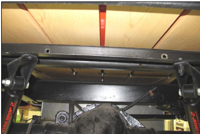
Front Tailpipe Hanger Frame Bracket Installation Figure 1
