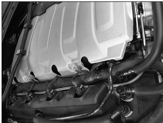
**Figure 13 – Fuel Line Routing**
