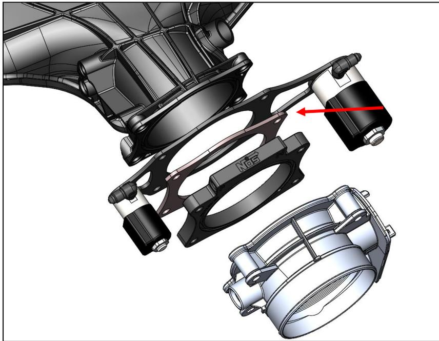
**Figure 9 – Nitrous Plate & Solenoid Bracket Installation**
