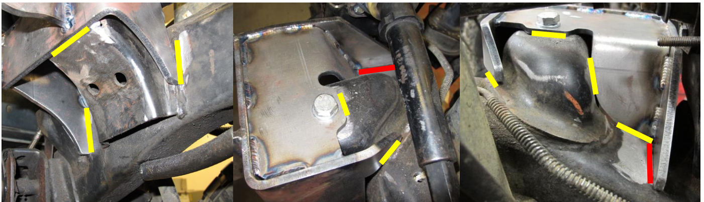
Image 7- minimum weld locations for the driver side engine mounting bracket
