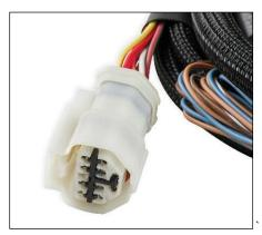
Figure 34 - Main Transmission Connector AODE/4R70W 92-97
