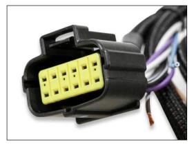
Figure 35 - Main Transmission Connector 4R70W/4R75W 98+
