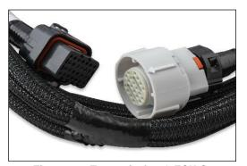
Figure 32 - Transmission & ECU Connector
