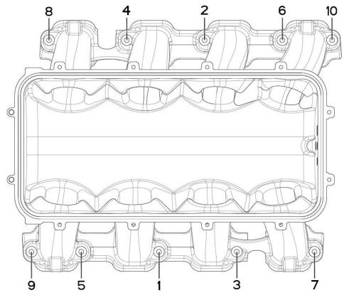
**Base Manifold Tightening Sequence**
