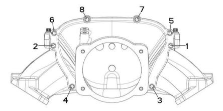
**Throttle Body Adapter Fastener Tightening Sequence**
