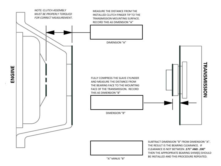
NOTE: All fasteners for the engine side or transmission side should be torqued between 35 and 45 ft./lbs. to maintain parallelism. It is more important that they are all torqued the same more than whether it is 35 or 45 ft /lbs.
